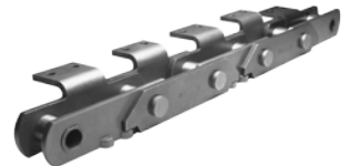
160mm pitch self supporting clinker tray conveyor chain w/ integral A2 attachment
