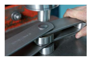
As specialists in the production of spin-riveted chains, we use high-grade case-hardened alloy steel pins produced on state-of-the-art European machines, giving you the best rivet on any standard chain.
